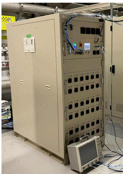
Figure 8: Actual photo of the amplifier for SCSS+.
