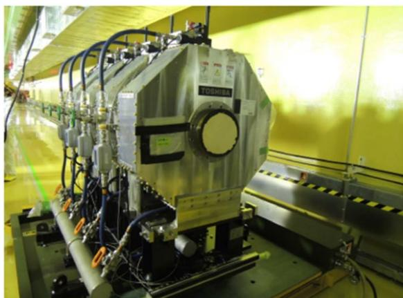
Figure 8: Installation work of the new RF cavity (single-ended cavity) at RCS in 2023 summer.
