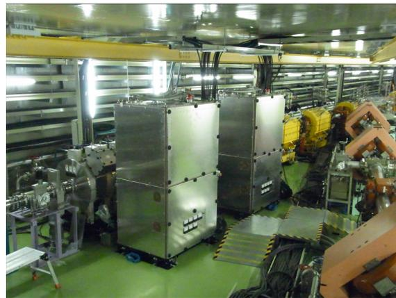
Figure 2: Two 2<sup>nd</sup> harmonic RF cavities with FT3M.
