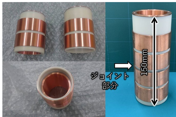
Figure 13: Picture of ABS resin + copper-plated insulation tube.
