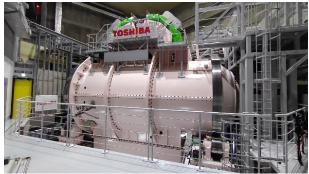
Figure 1: Rotating gantry for carbon ion radiotherapy with combined function superconducting magnets developed by Toshiba Energy Systems and Solutions installed at Yamagata University.
