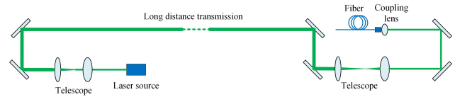
Figure 2: Experimental layout of the long-distance transmission experiment with transmission telescope.
