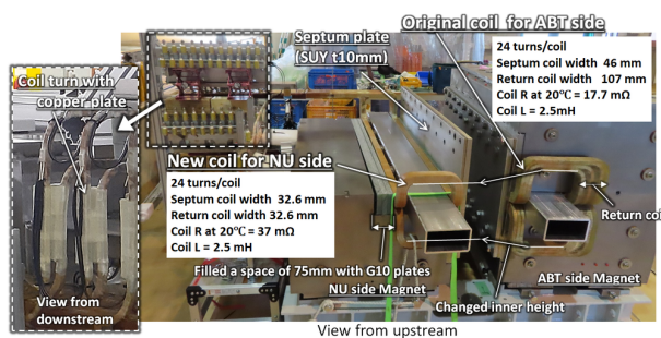
Figure 1: Photograph of new magnetic coil for NU side and original magnetic coil for ABT side.
