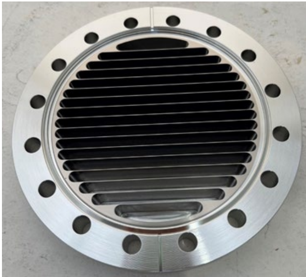
Figure 1: The ICF152 zero-length NEG pump fabricated by double deposition of oxygen-free Pd/Ti on a groove-machined ICF152 blank flange.
