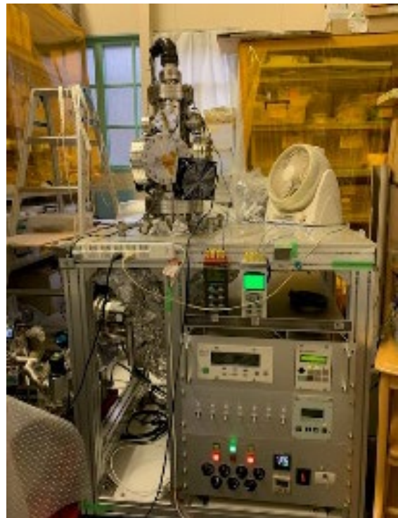
Figure 2: The evaporation equipment for oxygen-free Pd/Ti deposition.
