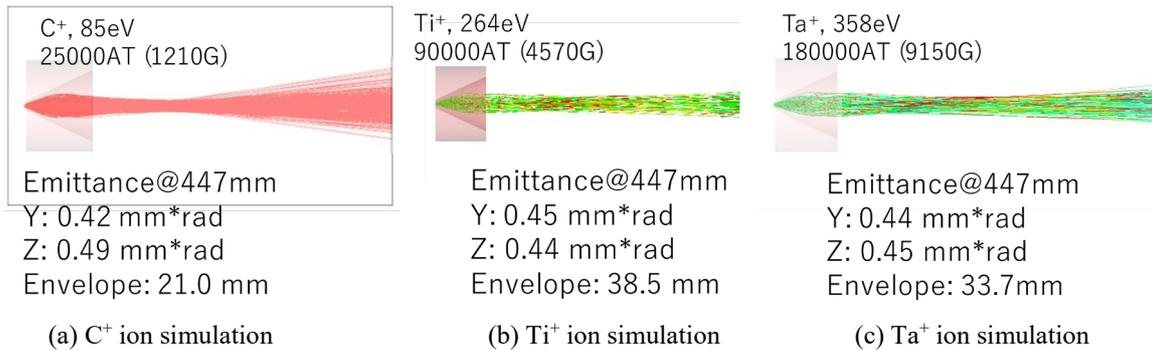
Figure 5: Simulation results of ion transport in the designed tapered solenoid.
