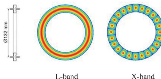
**Figure 1.** RF field distribution in the ring shaped cavity for the L- and X-band klystrons.
