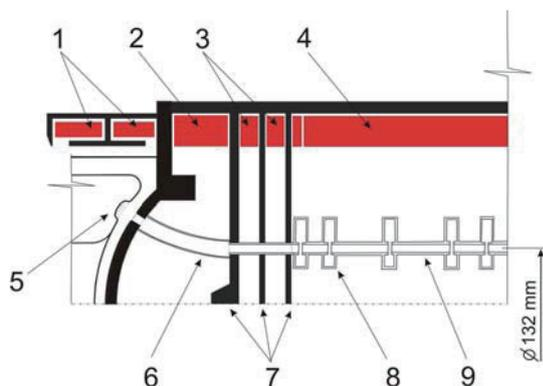
1. Cathode coils; 2. Compression lens coil; 3. Matching lens coils; 4. Solenoid; 5. Cathode; 6. Coaxial structure for beamlets transport; 7. Magnetic shield (material: steel); 8. Klystron cavity; 9. Individual drift tube for beamlet
