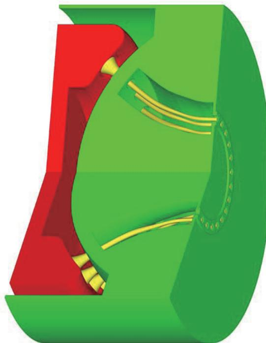
**Figure 3.** Example of the multiple beam gun modeling by using the GUN3D code (40 MW X-band klystron case)
