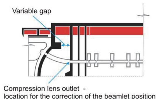
**Figure 6.** Displacements correction scheme.
