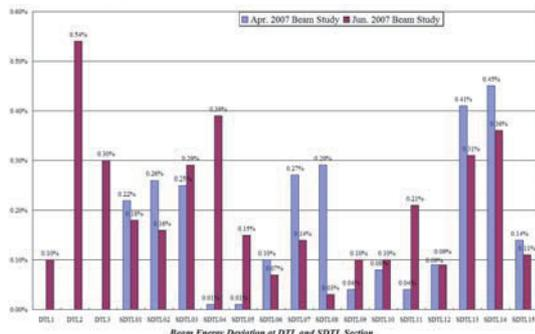
Figure 7: Energy Deviation in DTL and SDTL Section.
