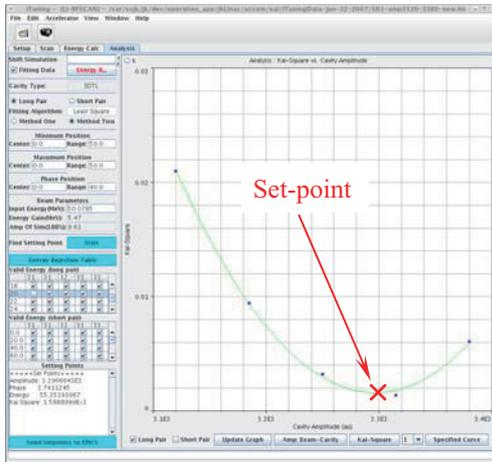
Figure 1: Signature Matching Error of SDTL01.
