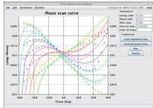
Figure 5: Comparing the measured curve with those from PARMILA modeling for DTL1. The marker is measurement, and the line is data from modeling shifted manually.
