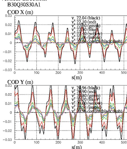
Figure4: The horizontal COD as a function of the longitudinal distance in one-third of the ring for  $\nu_x = 22.04 \sim 22.46$  and  $\nu_y = 20.8$  (top figure) and the vertical COD for  $\nu_y = 20.54 \sim 20.96$  and  $\nu_x = 22.4$  (bottom figure).
