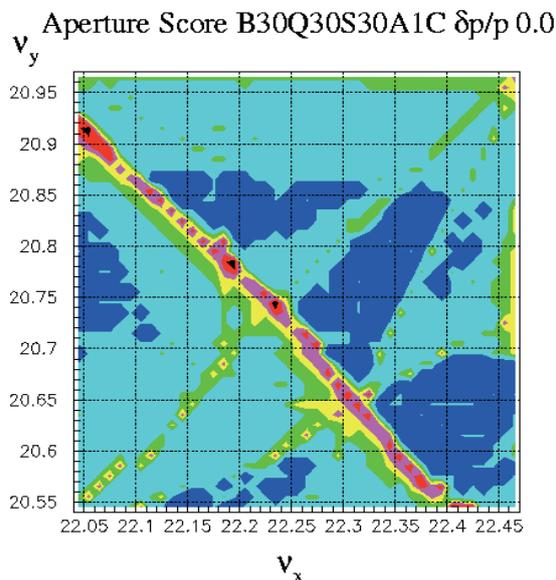
Figure 6: Available apertures are shown in each color for the horizontal tune of 22.04~22.46 and the vertical tune of 20.54~20.96. The color of the tune area is blue if a particle with the Courant-Snyder invariant of  $72.9\pi$  mmmrad is survived. The color of sky blue is for  $64.8\pi$ , green for  $56.7\pi$ , yellow for  $48.6\pi$ , pink for  $40.5\pi$ , red for  $32.4\pi$  and black for  $24.3\pi$  or less.
