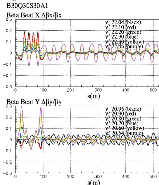
Figure 5: The horizontal  $\beta$  modulation as a function of the longitudinal distance in one-third of the ring for  $\nu_x = 22.04\sim 22.46$  and  $\nu_y = 20.8$  (top figure) and the vertical  $\beta$  modulation for  $\nu_y = 20.54\sim 20.96$  and  $\nu_x = 22.4$  (bottom figure).
