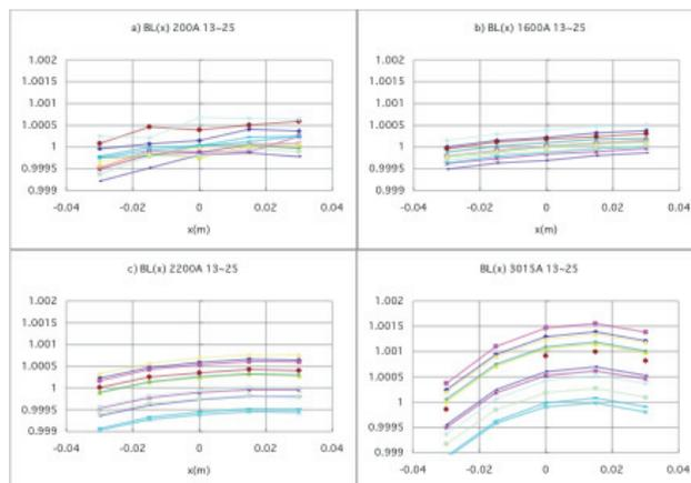
Figure1: Relative field integral as a function of the horizontal coordinate of 12 bending magnets for the corresponding energies of (a) 3GeV, (b) 30 GeV, (c) 40 GeV and (d) 50 GeV.
