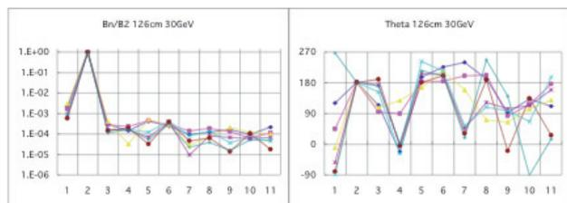
Figure3: The left figure shows seven time measurements of the relative amplitude of the multipole components of the reference quadrupole magnet for 30 GeV. The right figure shows seven time measurements of the phase of the multipole components of the reference quadrupole magnet.
