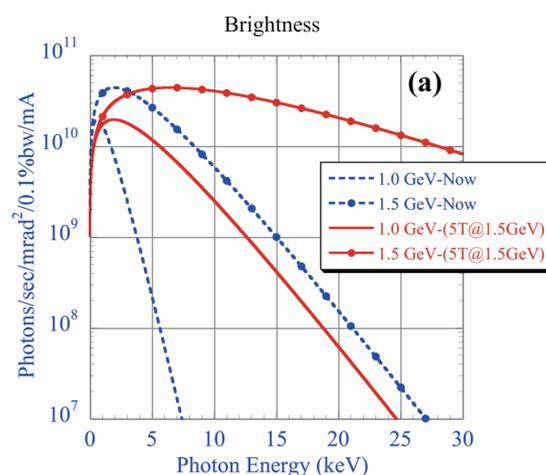
Fig. 1. Expected photon spectrum (brightness) for an electron beam current of 1 mA.
