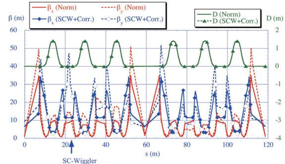
Fig. 6. Optics without/with SC wiggler ( $\theta$  is 0.3 rad). The latter is corrected by additional quadrupole magnets.
