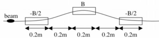
Fig. 4. SC wiggler composed of three superconducting magnets. Peak field strength is B for the central pole and  $-B/2$  for the compensating poles.
