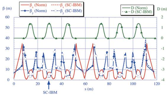
Fig. 3. Twiss parameters along the storage ring. Solid and broken lines indicate optics with the normal and the superconducting inverse bend, respectively.
