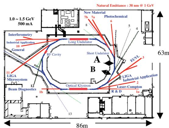
Fig. 2. Line drawing of NewSUBARU facility. A is the proposed position for superconducting IBM, and B is that for the superconducting wiggler.
