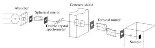
Fig. 7. Line drawing of beam line for radiation from the SC-IBM.
