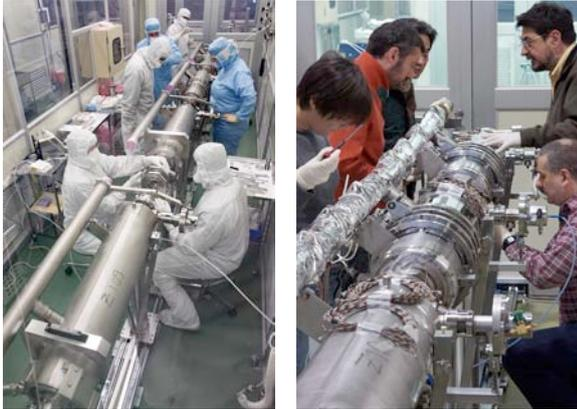
Fig. 2: Researchers from DESY, FNAL, and KEK working in clean room (left), team from INFN, FNAL, and KEK installing frequency tuners (right).
