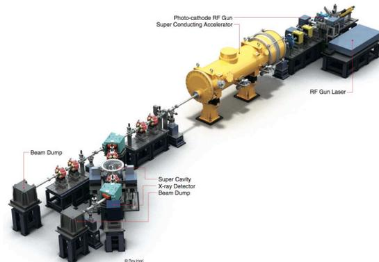
Fig. 9: Illustration of compact X-ray generation experiment setup, and later to be used for STF phase-2 beam source.
