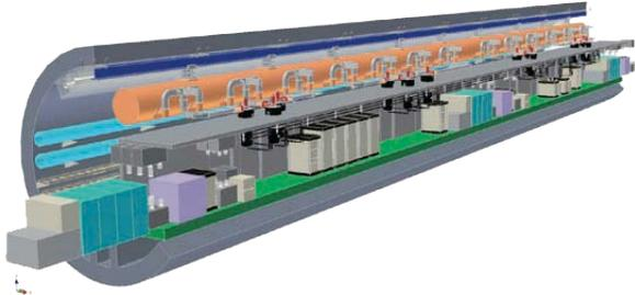
Fig. 6: Illustration of DRFS installation in the single tunnel design.
