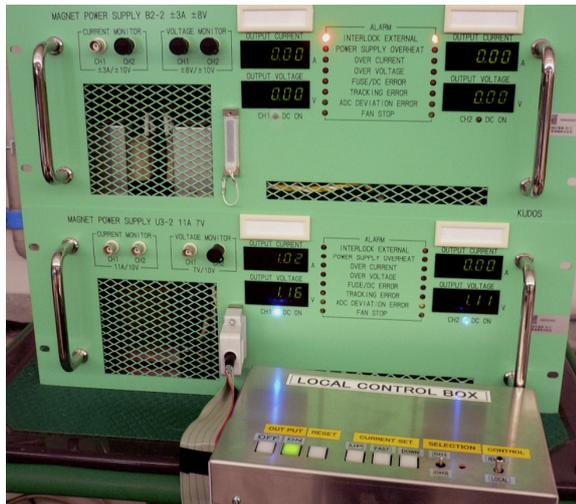
図13: Local Control Boxを繋いだ光源棟用小型電源
