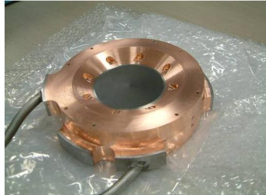
Figure 1: Picture of the fabricated muon target.
