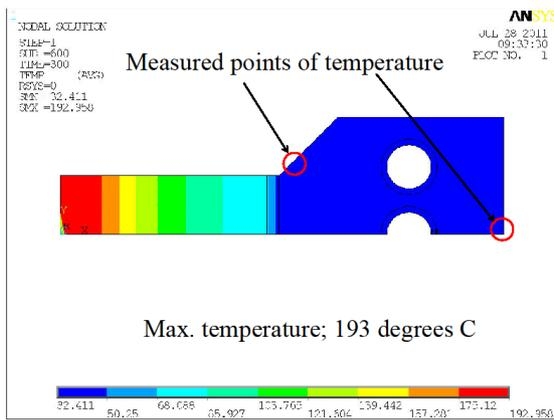
Figure 2: The temperature distribution of the muon target at  $t=300$  (s)
