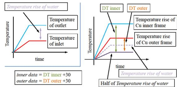
Figure 3: The explanation of the parameters used in this section
