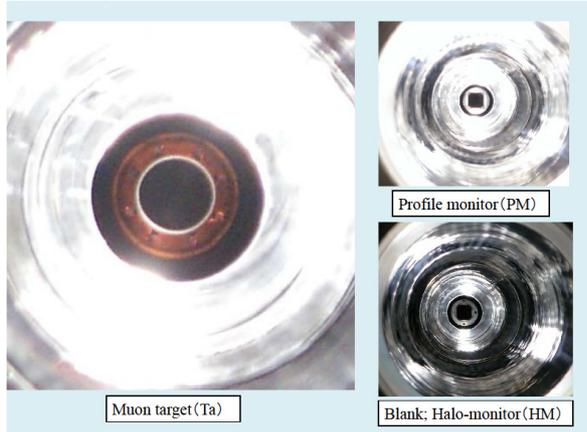
Figure 7: The taken pictures of the irradiated muon target, the profile monitor, and the halo-monitor
