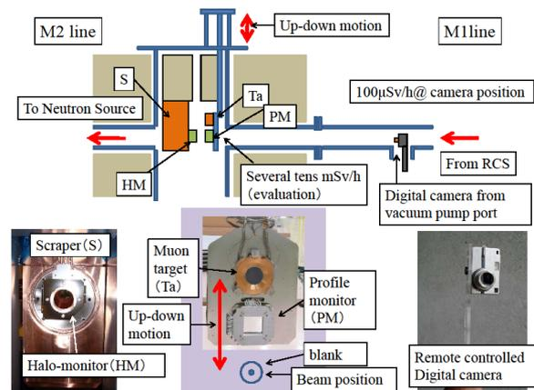
Figure 6: The schematic drawing of the observation for the muon target
