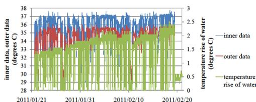
Figure 5: the variation in 500-seconds intervals of the temperature rise of the water and the temperature of the *inner data* and the *outer data*
