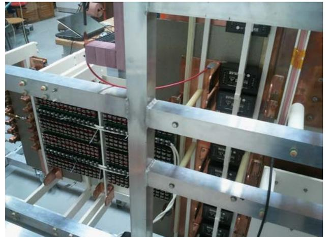
Figure 3: The HV switch in injection configuration.
