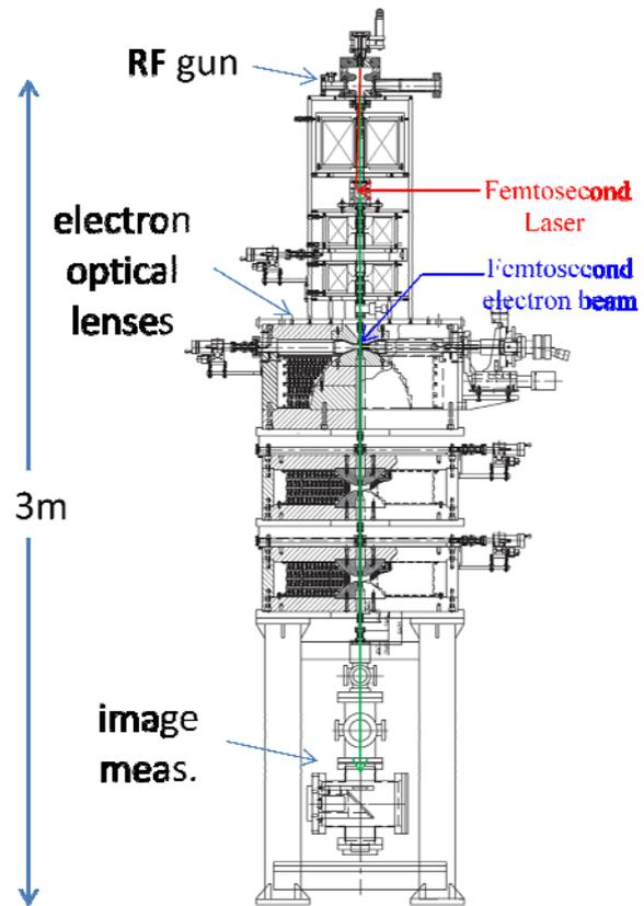
Figure 1: Concept of time-resolved relativistic transmission electron microscopy (TEM) using RF gun
