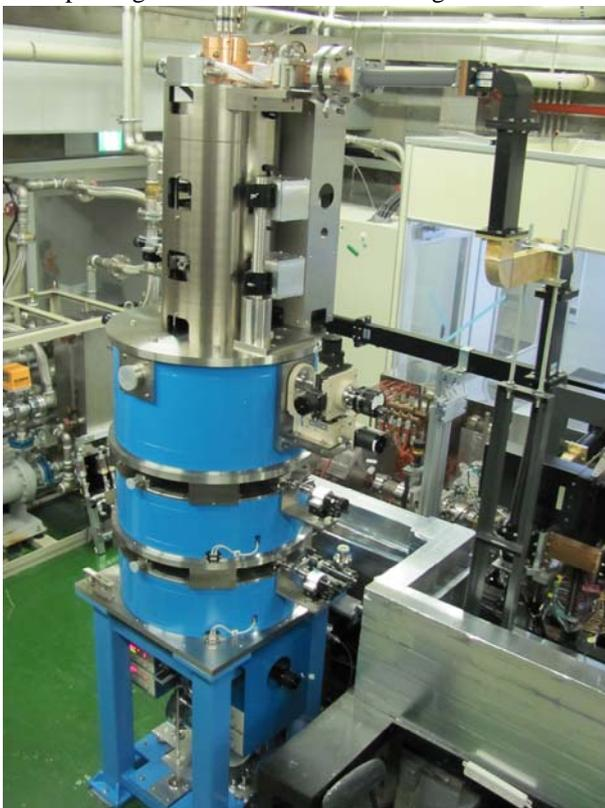
Figure 2: Prototype of RF gun based time-resolved relativistic TEM. The height is 3 m and the diameter is 0.7 m.
