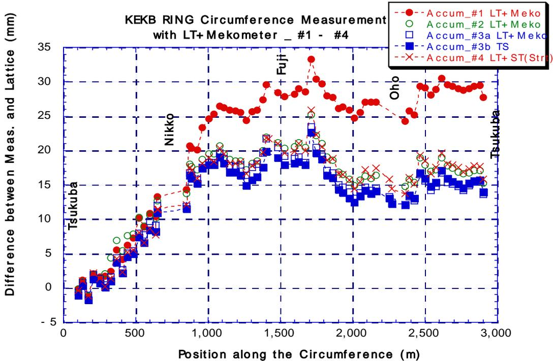
Figure 2: Accumulation of dL (difference between measurement and designed value)
