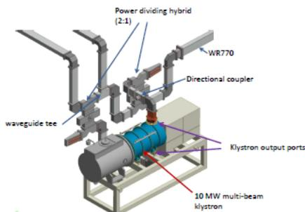
Figure 10: Klystron power system
