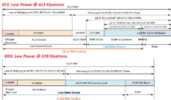
Figure 11: Power consumption comparison between KCS and DKS.
