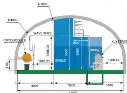
Figure 1: Cross section view of Kamaboko tunnel and layout of DKS.
