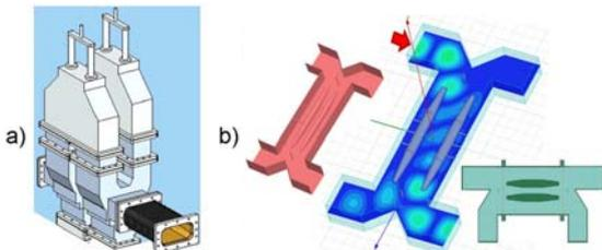
Figure 9: Tap-offs or variable hybrid (a) tap-offs with two folded magic-T's and two U-bend phase-shifters (b) variable H-hybrid with two moving conductor
