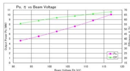
Figure 5: Characteristics of MBK, an output power and efficiency with the function of applied voltage.
