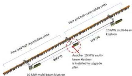
Figure 3: Bird-eye view of 6 cryomodules with two 10 MW MBKs and two LPDSs in the baseline
