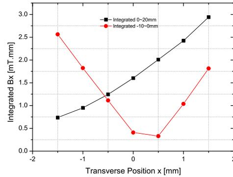
Figure 7: Integrated transverse magnetic field  $B_x$  along  $z$  for straight slit FC.
