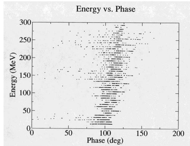
Figure 3: Phase drift of survival electrons until 50 turns (300 MeV) of acceleration with 6 MeV/turn.
