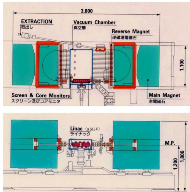
Figure 1: Cross sections of conventional 150 MeV RTM.
