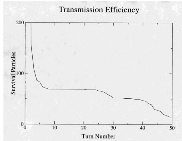
Figure 2: Transmission efficiency in the case of 300 MeV acceleration with 6 MeV/turn.
