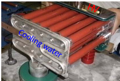
Figure 6: Cooling of matching resistor
