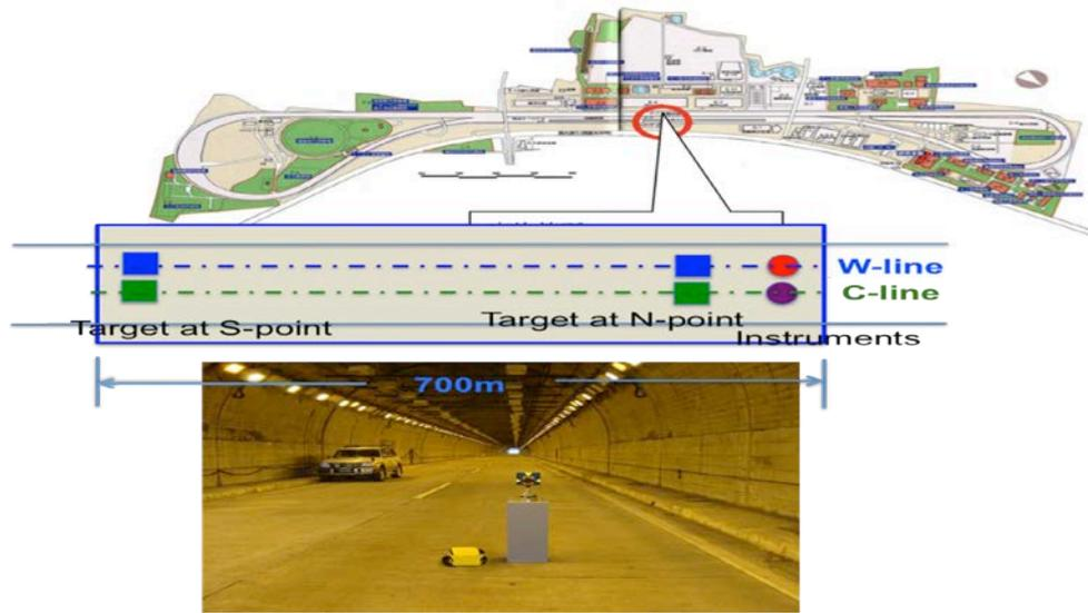
Figure 1: Layout of the test road, and the configuration and a picture for the test lines in 700 m long tunnel located in the center of the test road.
