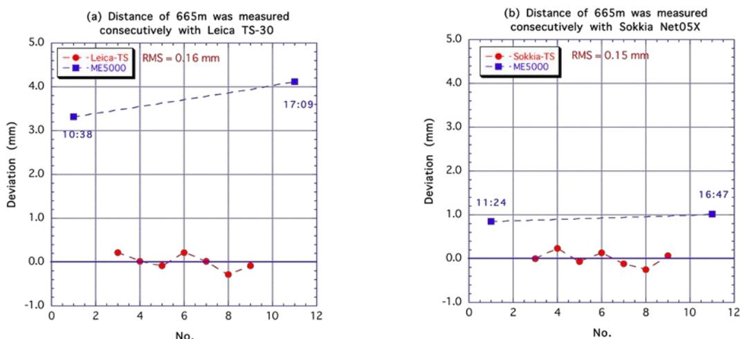
Figure 3: Variation of consecutive measurements of the distance 665m at one-hour time interval with (a) TS30 No.1 and (b) Net05X No.1.
