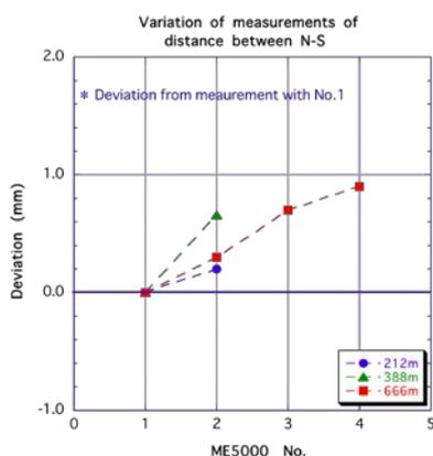
Figure 4: Differences among measurements of three distances, 212 m (blue points), 388 m (green points) and 666 m (red points), with two or four mekometers. The measurements with ME5000 No.1 are taken as the reference.
