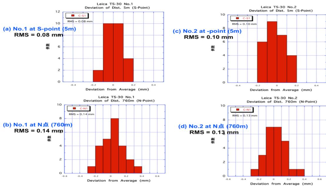
Figure 2: Deviations from the average value of 25 measurements for the same distance. (a) and (b) are those for 5 m and 760 m distances measured with TS30 No.1. (c) And (d) are those for TS30 No.2 measurement button successively.
