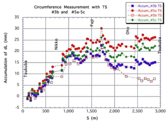
Figure 6: Accumulation of dL in the circumference measurements performed for December 7-9, 2011 (blue points) and in two weeks in June 2012 (other three color plots), where dL is the deviation of the distance measurement from the designed value in each measurement stage.
