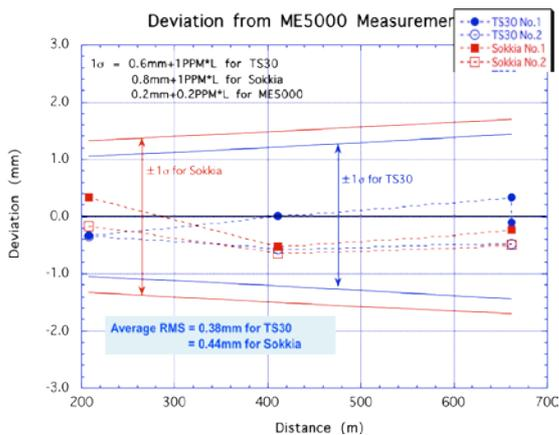
Figure 5: Deviations of measurements for three distances, 208 m, 411 m and 662 m, with TS30 and Net05X from those with ME5000 No.1. Blue plots are for TS30 No.1 and No.2, and red plots for Net05X No.1 and No.2.
