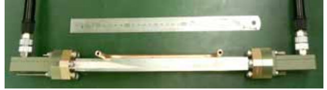
Figure 1: Narrow waveguide of stainless-steel (#SUS003).
