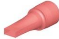
Fig. 2: Schematic of mode converter
