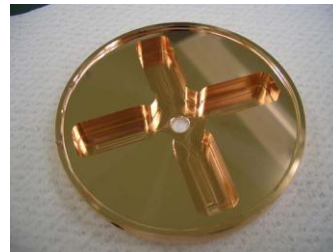
Figure 2: Typical damped cell of TD18 structure.
