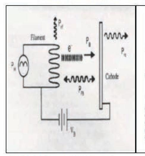
Schematic view of an indirectly heated cathode model
