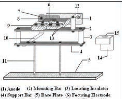
(4) Support Bar (5) Base Plate (6) Focusing Electrode
