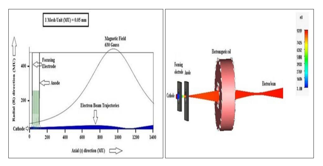
Two dimensional (2-D) Plot of beam trajectories.
