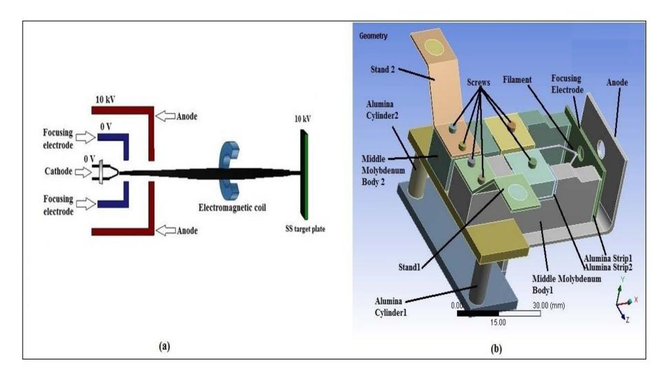
(a) Two dimensional schematic view of the gun with electromagnetic coil and target, and (b) Three dimensional model of the gun.
