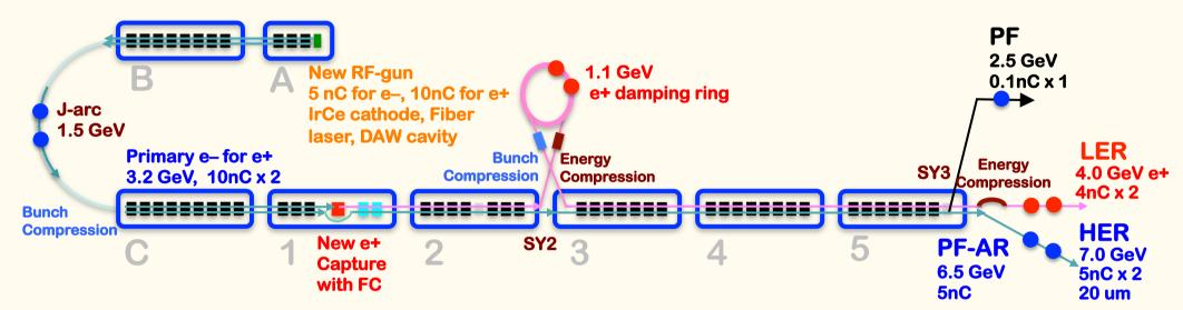
As a high-field (several Tesla) pulsed solenoid for the positron source of the SuperKEKB injector, KEK is going to fabricate a SLAC-type flux concentrator.
