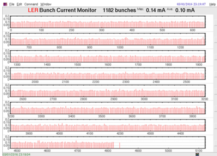
Figure 13.13: Bunch Currents at LER after turning on BCE: the BCE operation is turned on just after we take data in Figure 13.12. These data are taken 13 minutes later that. The bunch currents are fairly equalized.
