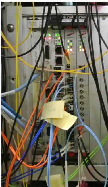
Figure 13.7: Picture of MR-STs IOC: the EVG and EVR modules developed at SINAP is installed in the VME type EPICS IOC. The EVG delivers new Events when it receives Events from MTS. They are delivered to the EVR installed in the next slot and those installed at D7 and D8.
