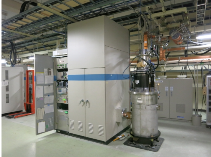
Figure 11.23: Overall view of the compact modulator with the klystron assembly and the SLED cavity.
