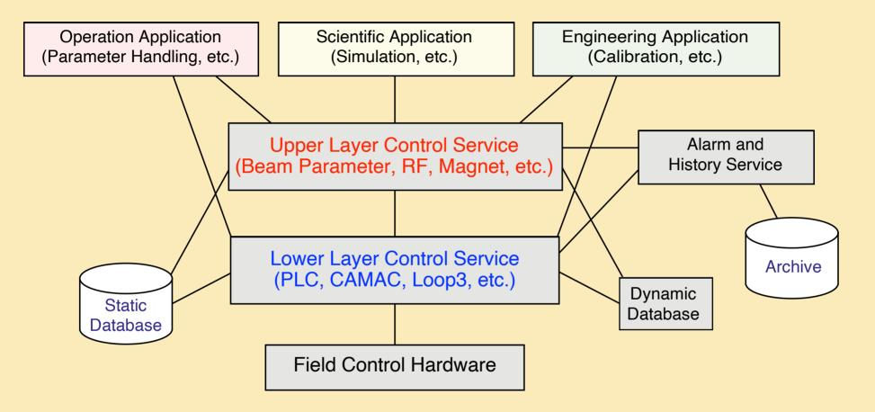
Each lower layer software supports corresponding field controllers. Upper layer software hide differences between controllers and serves accelerator equipment controls to clients. While UDP-based RPC protocol is used at lower layer, upper layer make use of TCP-based one.
