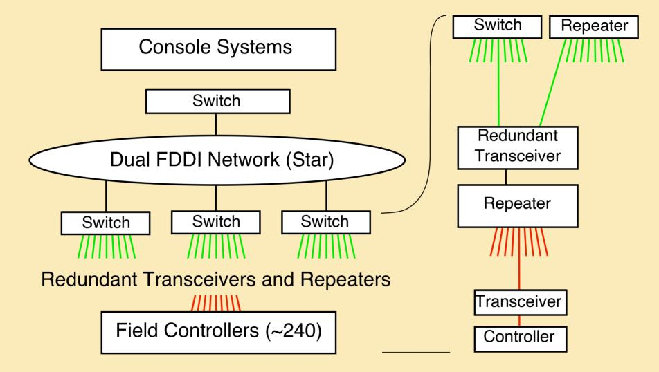
33 field network stations are connected with central switches on FDDI through redundant 10Base-FL Ethernet. Each station is connected to 4 to 10 field controllers. All connections at fields use 10Base-FL because of the klystron noises. Network traffic at important points are monitored via SNMP.
