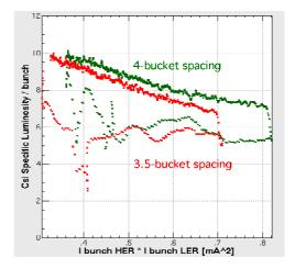
Figure 6: Specific luminosity in 3.5-bucket spacing operation.
