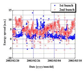
Fig. 5: Result of long-term mesasurement. Filled circle (blue) and open circle (red) show the energy spread of 1st and 2nd bunch respectively.
