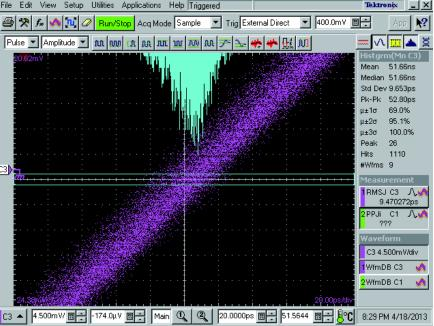
After collecting 1000 samples, timing and its jitter is determined from center value and standard deviation of distribution.
