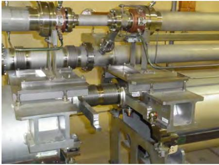
Figure 3: Mechanical jigs for mounting the tracker target. The jig and QPD are connected by high-precision flange-flange mechanical joining.
