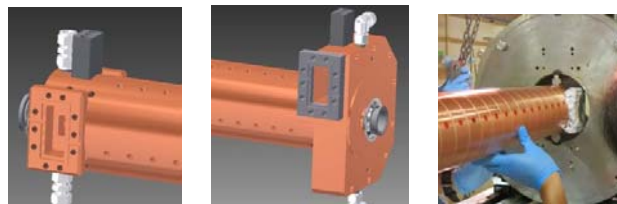
Figure 3: LAS output end (left), input end (center) and insertion of LAS into solenoid (right).
