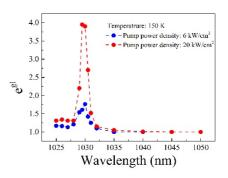
Figure 9: Gain test for different seed laser wavelength at 150 K under different pump power density.
