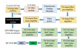
Figure 1: Layout of laser system.
