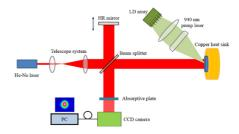
Figure 4: Optical measurement experimental setup.
