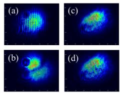
Figure 5: Optical measurement results for thermal effect. (a) and (b) are measured by use of old design; (c) and (d) are for Yb:YAG/Cu composite.
