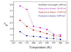
Figure 8: Gain test under different pump power density for 1030 nm seed laser at different temperature.
