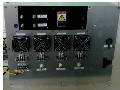
Figure4: Photograph of one Chopper-type Marx unit.
