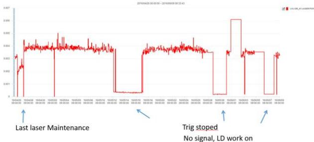
Figure 2: Stability of Laser system from 4/26 to 6/9.
