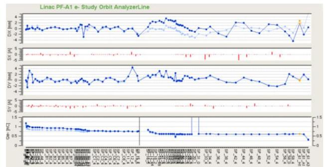
Figure 3: 2 bunches beam transport orbit and charge
