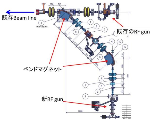
Figure 5: 90 deg injection line
