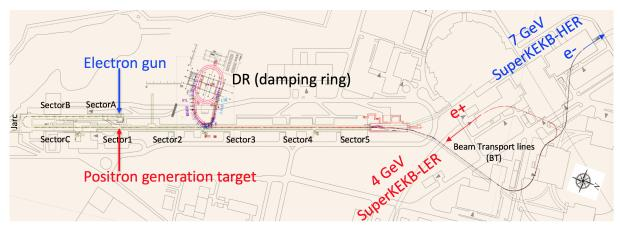
Figure 2: A footprint of SuperKEKB injector LINAC and the beam transport line.
