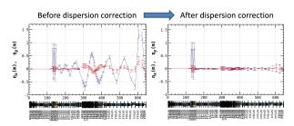
Figure 3: Dispersion measurement before and after the dispersion correction in the LINAC.
