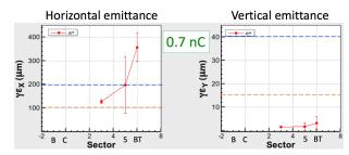
Figure 12: Emittance measurement result for positron beam at each sector.
