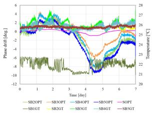
Figure 5: Long-term phase drift of the reference phase and the temperature fluctuations in the klystron gallery.
