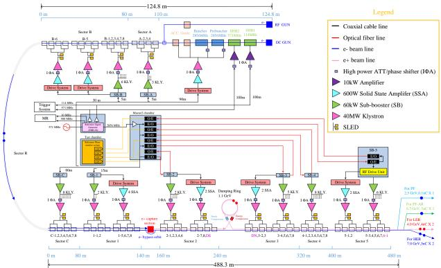
Figure 1: Layout of the RF reference distribution for the SuperKEKB Injector LINAC.
