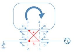
Figure 2: Schematic diagram of the resonant ring.
