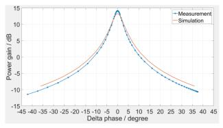
Figure 6: Measured and simulated power gain compared with one-turn phase drift.
