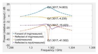
Figure 9: Measured responses of fully tuned resonant ring with input of 500 W.
