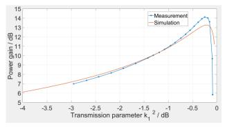
Figure 5: Measured and simulated power gain compared with transmitted coefficient  $k_{1}^2$
