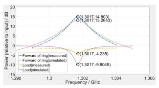
Figure 8: Measured and simulated responses of fully tuned resonant ring with input of 500 W.
