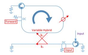
Figure 3: Structure diagram of the resonant ring.
