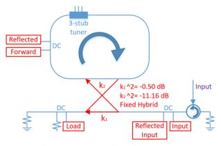
Figure 7: Resonant ring with 3-stub tuner.
