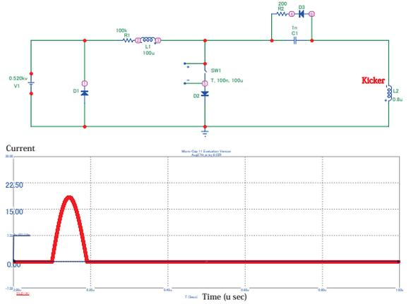
Figure 7: Top: The schematic electronic circuit for the pulsed magnetic kicker. Bottom: The pulsed current through kicker coil.
