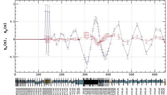
Figure 4: Dispersion measurement before the dispersion suppression.
