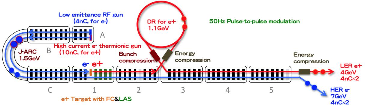
Figure 1: Schematic layout of the SuperKEKB injector linac.
