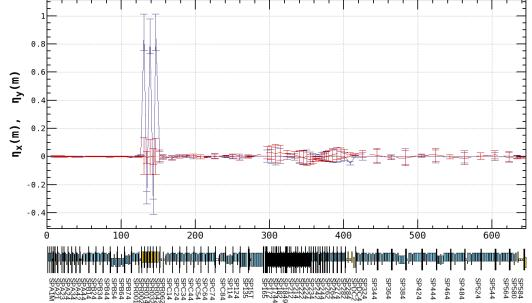
Figure 5: Dispersion measurement after the dispersion suppression.
