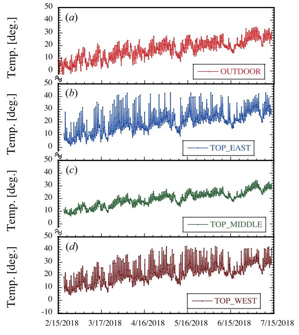
Figure 7: Time traces of environmental temperature measured at (a) the outdoor, (b) the top floor (east), (c) the top floor (middle), and (d) the top floor (west) of the linac building during the short term Feb.19-July.13.2018.
