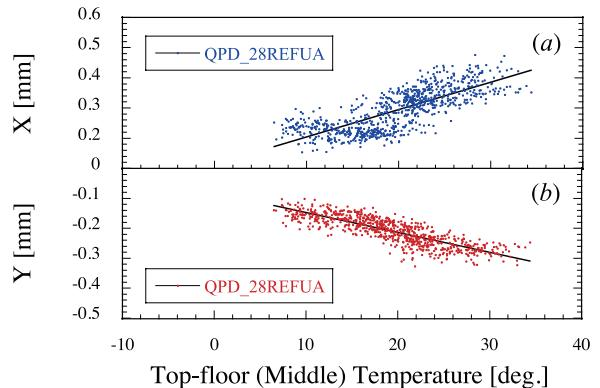
Figure 8: Correlation plots in the transverse displacement measurement of QPD\_28REFUA versus environmental temperature measured at the top floor (middle) of the linac building during the short term Feb.19-July.13.2018. (a) and (b) show the correlation plots in the  $x$  and  $y$  displacement measurements, respectively.
