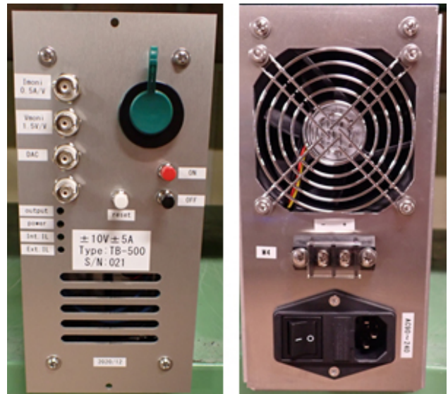
Figure 3: Front and back panel of the power supply. RJ45 connector is covered by the green rubber.
