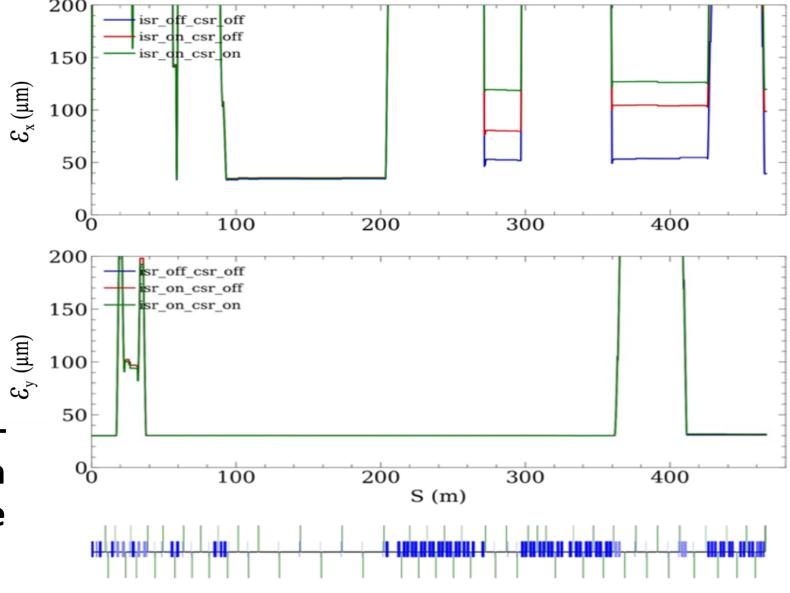
Figure 4: Evolution of the normalized horizontal (top) and vertical (bottom) emittances along the beam transport.
