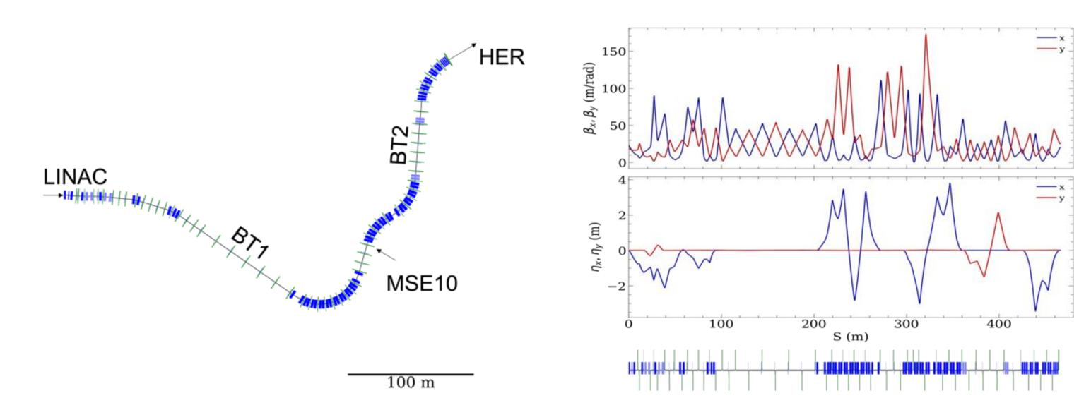
Figure 1: 7-GeV electron beam transport between the SuperKEKB high-energy ring (HER) and the LINAC.
