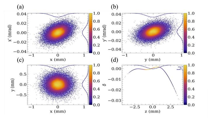
Figure 3: Initial beam distribution on the (a) x– x', (b) y–y', (c) x–y, and (d) z– $\delta$  planes, with normalized histograms in dark-blue before the 7-GeV electron beam transport.
