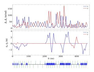
Figure 2: Nominal 7-GeV electron beam transport optics with dispersion functions shown in blue and red for the horizontal and vertical directions, respectively.
