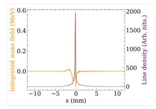
Figure 6: Longitudinal charge profiles (purple) and integrated CSR wake field produced by a bending magnet (orange) in Arc1.
