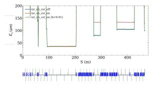
Figure 10: Evolution of the normalized horizontal emittances with narrower beam duct. The normalized horizontal emittances at the injection point 1) with ISR (blue), 2) with ISR and CSR (red), and 3) with ISR and CSR and a duct height of 10 mm (green) are 99, 126, and 100  $\mu$ m, respectively.
