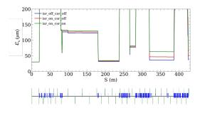
Figure 9: Evolution of the normalized horizontal emittances. The normalized horizontal emittances at the injection point 1) without ISR and CSR, 2) with ISR, and 3) with ISR and CSR are 38, 52, and 66  $\mu$ m, respectively.
