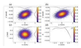
Figure 3: Initial beam distribution on the (a) x-x', (b) y-y', (c) x-y, and (d)  $z-\delta$  planes, with normalized histograms in dark-blue before the 7-GeV electron beam transport. The color code indicates the density of the beam.
