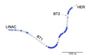
Figure 1: 7-GeV electron beam transport between the SuperKEKB high-energy ring (HER) and the LINAC. It comprises two achromatic sections of BT1 and BT2. The bending and quadrupole magnets are indicated in blue and green, respectively.
